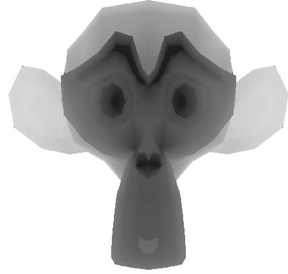
Figure 6. Ecce Mono. Our simple ray tracer, driven entirely by TTU instructions in compute mode, produces a monkey model [2]. Each pixel is colored according to the depth returned by the TTU.
