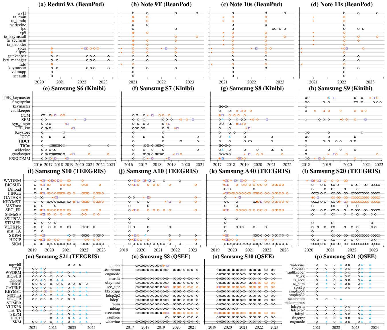
Figure 9: The TA vulnerability lifecycle for TAs found on 16 devices covering the four most widely-used TEE implementations. A circle \circ represents an update to the TA. A \times represents a vulnerability. A square \square represents a published advisory. A triangle \triangle represents an update with a rollback counter increase. Orange circles \circ are updates to a vulnerable TA that do not increase the rollback counter. If the last update to a TA is marked with an orange circle, then a vulnerable version of that TA may be loaded on the latest firmware of that phone.
