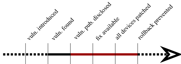
Figure 2: The TA vulnerability lifecycle. Attackers can leverage publicly disclosed vulnerabilities up until the rollback to a vulnerable TA version is prevented.
