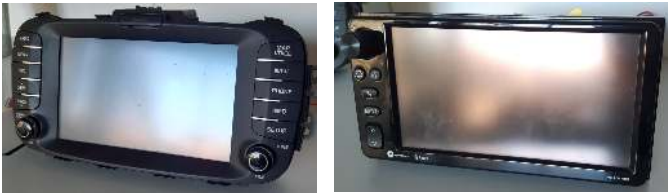
Fig. 3: Two of the five Bluetooth infotainment modules that we tested: a KIA 96560-B2211CA unit (on the left) and a Toyota PT546-00170 unit (on the right).
