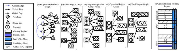
Figure 4: Compartment creation process and the resulting memory layout. (a) PDG is transformed to an initial region graph (b). A compartmentalization policy is applied (c), followed by optimizations (d) and lowering to produce the final region graph (e). Which, is mapped to a compartmented memory layout with associated MPU regions (f).
