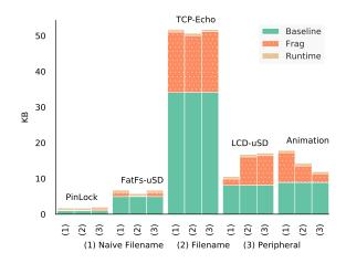
Figure 7: RAM usage of ACES for test applications
