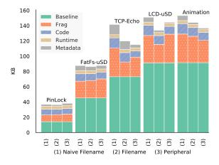
Figure 6: Flash usage of ACES for test applications
