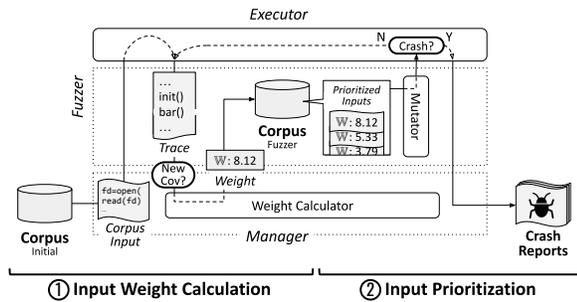
Figure 7: Design of SyzRisk runtime components.
