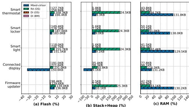
Fig. 6. Summary of BenchIoT memory utilization metrics for  $\mu$ Visor, Remote Attestation (RA), and Data Integrity (DI) defense mechanisms overhead as a % over the baseline applications. The size in KB is shown above each bar.
