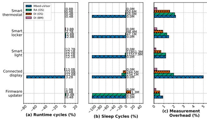
Fig. 5. Summary of BenchIoT performance metrics for  $\mu$ Visor, Remote Attestation, (RA) and Data Integrity (DI) defense mechanisms overhead as a % of the baseline insecure applications. BM: Bare-Metal.
