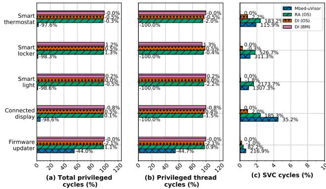
Fig. 7. Summary of BenchIoT comparison of minimizing privileged execution cycles for Mbed- $\mu$ Visor, Remote Attestation (RA) and Data Integrity (DI) defense mechanisms as a % w.r.t the total runtime execution cycles. The overhead as a % of the baseline insecure applications is shown above each bar. BM: Bare-Metal
