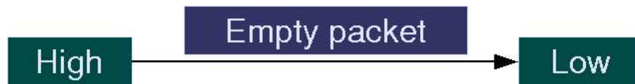
Figure 4.1: When a layer is registered, it has to pass a pointer to a free buffer to the lower layer.
