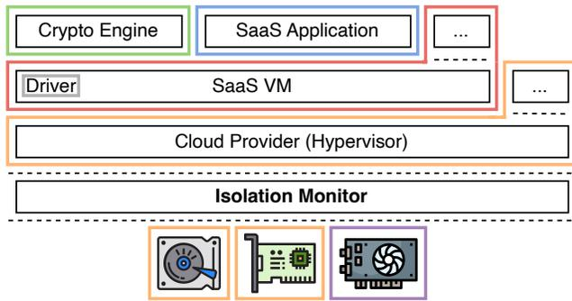
Figure 3: Deployment of Figure 2 on an isolation monitor. Black boxes denotes traditional system abstractions (hypervisor, VM, and processes), while colored boxes represent trust domains.
