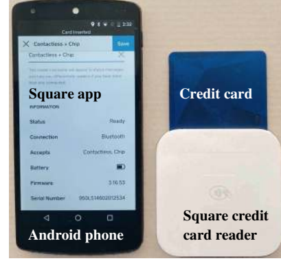
Figure 3: The Square app on Android phone with debloated Bluetooth stack communicates with the Square credit card reader.
