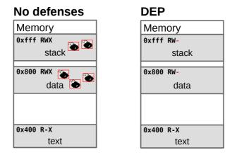
Figure 6.1: Changes to the address space of a process for DE-P/W^X. Bombs show memory areas an exploit may modify.
