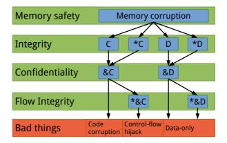
Figure 5.2: The attack flow of memory corruption-based attacks. 'C' conforms to Code, 'D' to Data; '&' marks an address-of operator; '\*' marks a dereference operator. The attack path needs to bypass defenses at different levels of abstraction: integrity, confidentiality, and flow integrity.
