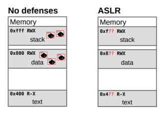
Figure 6.2: Changes to the address space of a process under ASLR.
