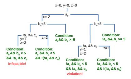
Constraint tracking along the different paths for the symbolic execution example.
